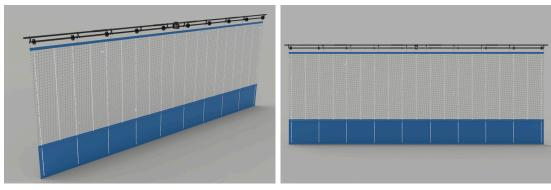
The lower section of the curtain is made from PVC, while the top section features a sturdy net design. A powerful motor, which is positioned at the top center, drives the system effortlessly. A tape mechanism smoothly opens the curtain, and a bottom counterweight ensures the canvas remains taut and stable when hanging.
