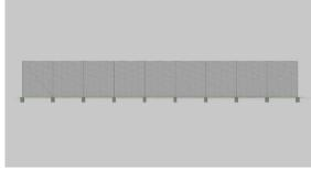
The backstop is made from high-grade aluminium profiles. The posts are fitted in ground sockets and measures a 120mm x 100mm x 2.5mm cross section. The net is made from high tenacity knotless PP and is fixed onto stainless steel wires that can be fixed with turnbuckles.
