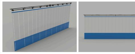
The lower section of the curtain is made from PVC, while the top section features a sturdy net design. A powerful motor, which is positioned at the top center, drives the system effortlessly. A tape mechanism smoothly opens the curtain, and a bottom counterweight ensures the canvas remains taut and stable when hanging.
