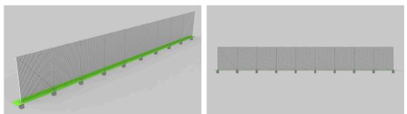
The backstop is made from high-grade aluminium profiles. The posts are fitted in ground sockets and measures a 120mm x 100mm x 2.5mm cross section. The net is made from high tenacity knotless PP and is fixed onto stainless steel wires that can be fixed with turnbuckles.
