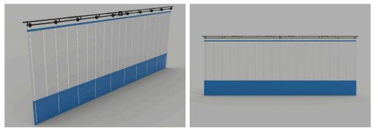
The lower section of the curtain is made from PVC, while the top section features a sturdy net design. A powerful motor, which is positioned at the top center, drives the system effortlessly. A tape mechanism smoothly opens the curtain, and a bottom counterweight ensures the canvas remains taut and stable when hanging.
